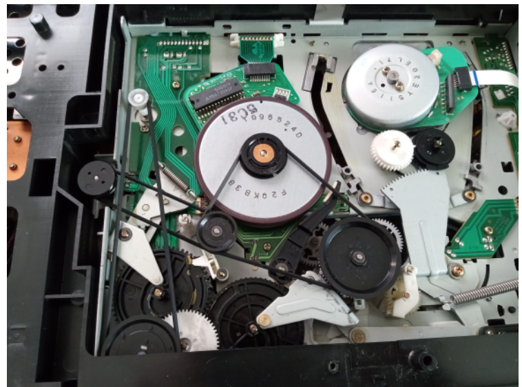
[New set of belts that drive the loading, unloading, and playback functions of the VCR.]
