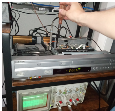
[Calibrating the VCR to match the tape. The oscilloscope image on the right shows 3 scan-lines on the tape and a nice balanced RF signal.]
