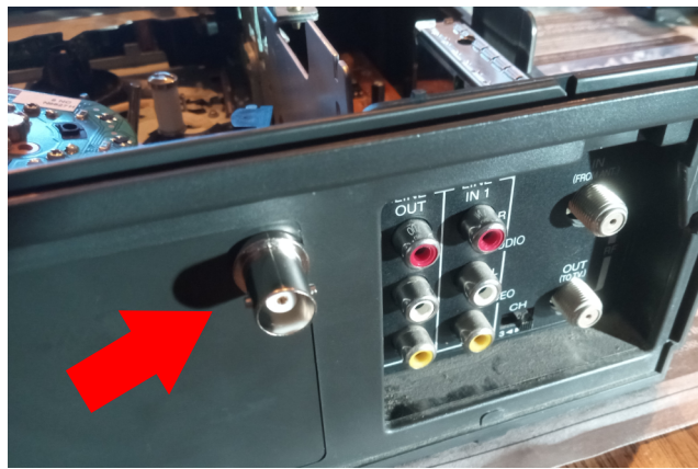
[VCRs need to have a RF tap. This "improved" VCR has a BNC connector added to the back which connects to the RF test point. The VCR drum reads data off the tape using the two heads on the drum, combines the signal from those two heads, amplifies it slightly, and makes it available on the RF test point. The small blue capacitor smooths out the signal.]
