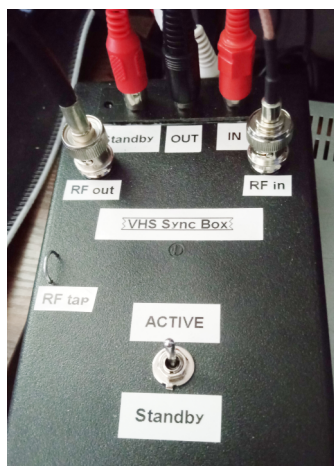
[You'll need a way to synchronize the sound to the video. I built this box around a two-pole switch. At the same instant, the RF signal is turned on and the sound goes from the Standby test tone to the VCR audio. This is critical to easily put the sound and video in sync at the beginning.]
