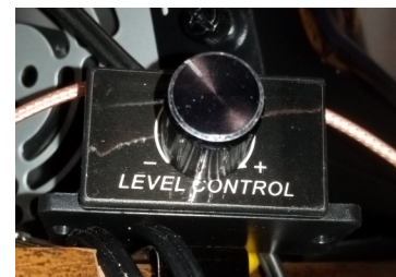
[An external volume control is handy. I found that loud segments could easily clip the line input of my sound card.]
